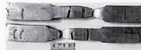
Figure 2: Close up views of the two tensile tested samples reveal that fracture occurred in base metal away from weld zone which confirming good quality of the welded joint.
